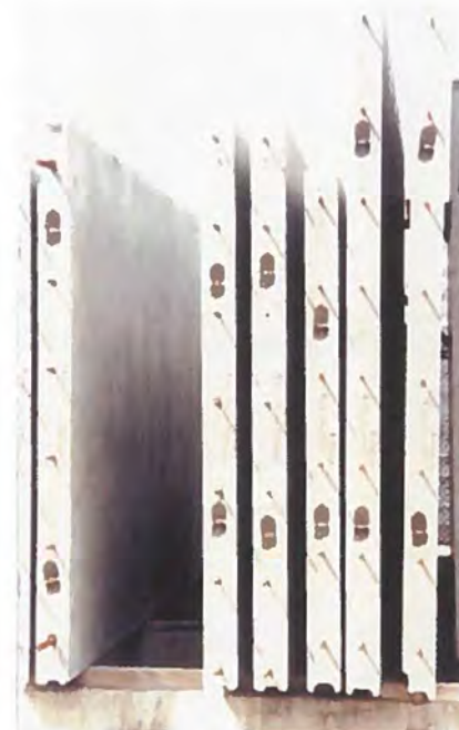
Internal walls by battery casting have high quality surfaces on both sides - no plastering is needed.
