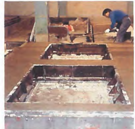
Top: Casting in a mould and finish of the topside.
