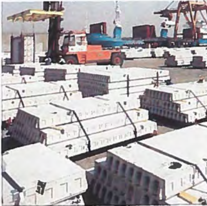
Top and Right: Continuous slab moulds where any length of slab components can be produced by flexible bulkheads.
