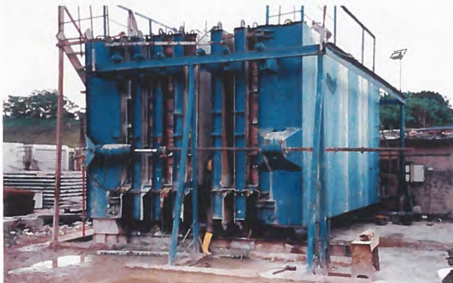
Internal walls by battery casting have high quality surfaces on both sides - no plastering is needed.
