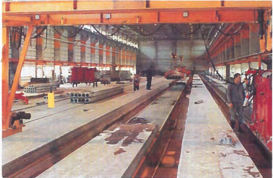
Top and Right: Continuous slab moulds where any length of slab components can be produced by flexible bulkheads.
