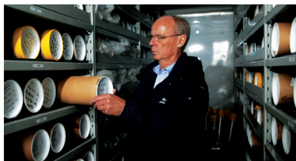
The soil samples taken from 50-100 m below the seabed are stored in container under controlled climatic conditions. Photo: Femern A/S
