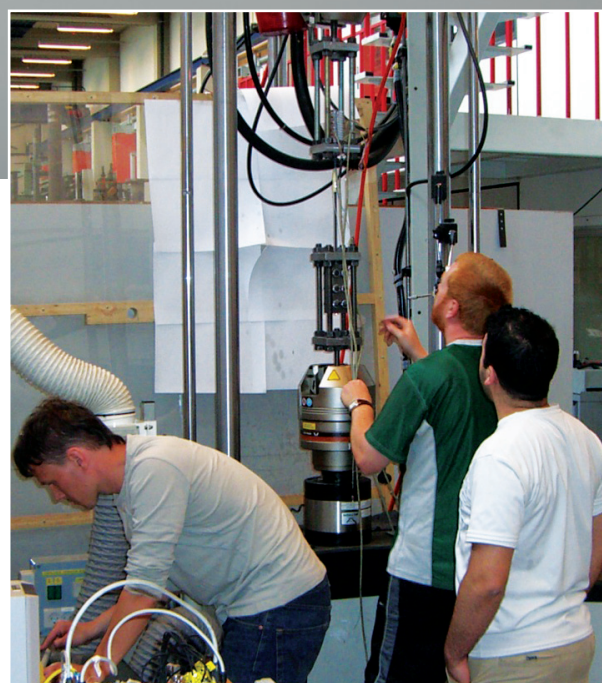
Testing the new anchor as part of a Master's project at DTU Civil Engineering. Photo: Jacob W. Schmidt
