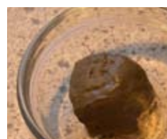
Example of a sensitive clay deposit which has a water content above the liquidation limit after thawing
