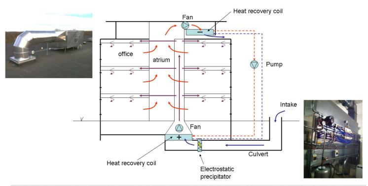
The heat exchanger coils are made from plastic tubing with extremely low obstruction to the airflow. Because of the use of cheap plastic tubing it is possible to have very large heat transfer area, something which is necessary to achieve high heat recovery efficiency. One exchanger has more than 5 km of plastic tubing inside.
