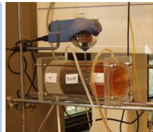
Fig 3: Picture and schematic diagram of electro dialytic treatment. The material to be treated is placed in compartment II. If the material is fine grained enough it can be treated in a homogenous suspension illustrated by the overhead stirrer.
