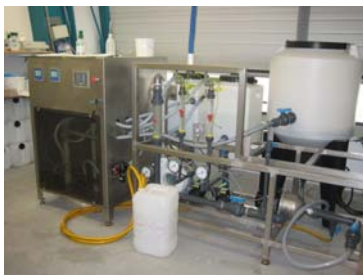
Fig 4: Pilot scale setup developed at DTU Byg for investigation of continuous treatment of various fine grained materials.
